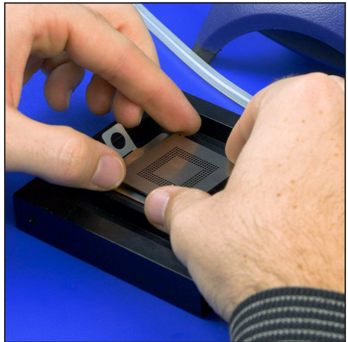
Figure 7. Placing the reball screen onto the component and aligning the apertures to the component pads
