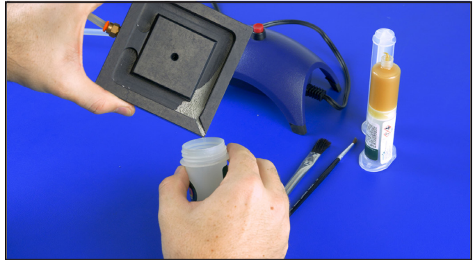
Figure 11. Pouring excess solder balls into a container
