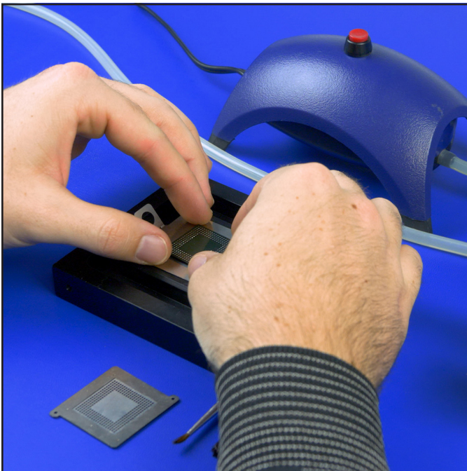
Figure 5. Placing the BGA component on the transfer plate over the vacuum hole
