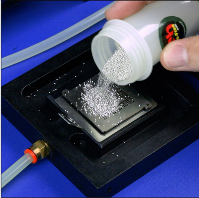
Figure 8. Pouring solder balls onto the reball screen
