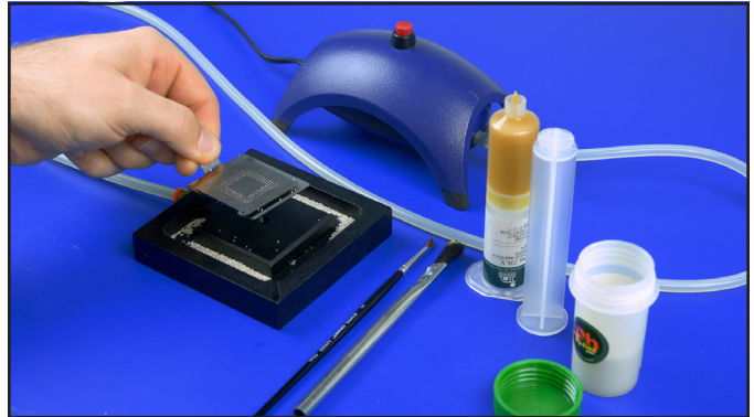
Figure 10. Lifting the component and reball screen using the transfer plate's handle
