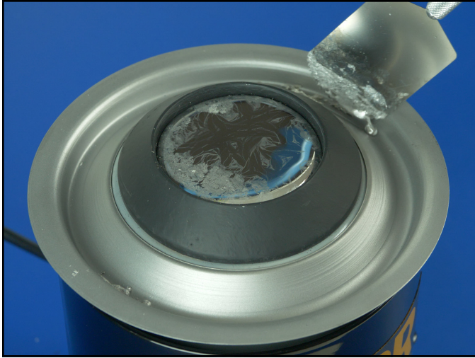
Figure 6. Placing solder dross onto the solder dross tray
